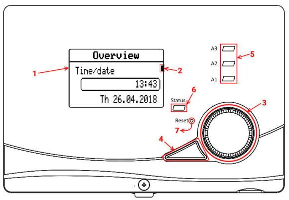
The display (1) on the front shows information about sensor measurements, menu position, parameters and such.
