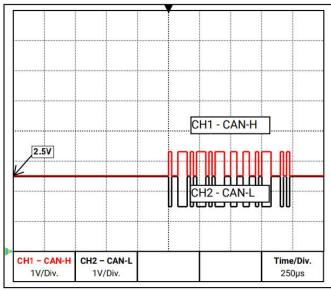
The CAN BUS comprises the cables CAN-High, CAN-Low, GND and one +12 V supply cable for bus components without their own power supply. The combined total load of all devices with 12 V and 24 V supply must not exceed 6 W.
