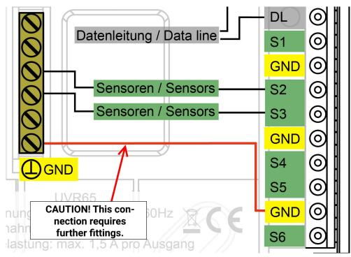
Sensors are always connected across the relevant sensor terminal (S1 – S6) and sensor earth (GND). There is an earth strip in the base. A connection to the GND terminal must be laid using this strip before the sensors are connected.
