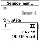
In the sensor menu, below the settings and measurements of all sensors, the setting **Simulation** is found.
