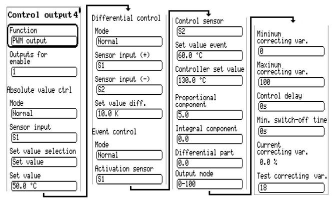
In most heating circuit programs, the two control outputs are already used to control the mixer and can therefore not be used for other applications.
