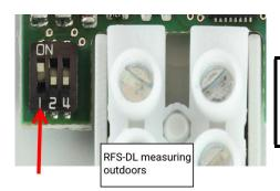
The RFS-DL intended to measure **outdoors** must have its DL-Bus address adjusted. **Dip-switch 1** must be set to **ON**. This changes the sensor's address to **2**.
