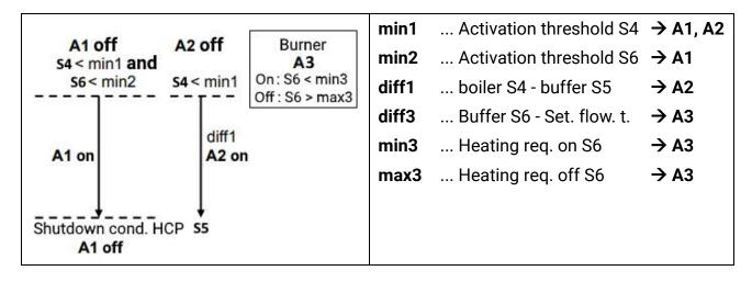
A1 = (S4 > min1 or S6 > min2) & (Heating = active) A2 = S4 > min1 & S4 > S5 + diff1 A3 on = S6 < min3 A3 off = S6 > max3 A4/A5 = Mixer Program 833: The burner is regulated only via S5.
