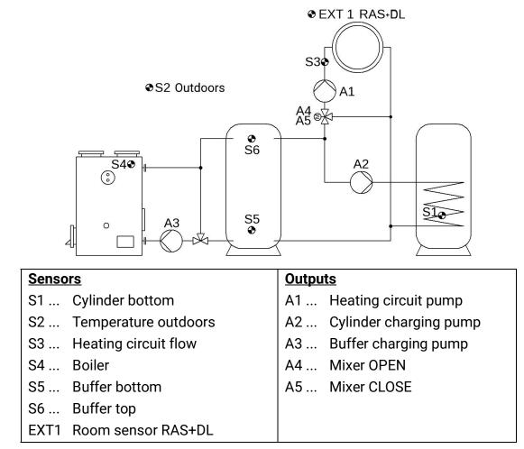
**Basic functions (P944):** Clearance for the heating circuit pump **A1**, if either the boiler's or the buffer's temperature has exceeded its respective minimum threshold, regulation of the cylinder charging pump **A2**, mixer regulation **A4+A5**, regulation of the buffer charging pump **A3**. The room sensor at EXT1 is intended to be an **RAS+DL** (not included).
