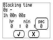
If an output is deactivated by usual automatic regulation, the blocking time must elapse before the output may be reactivated. Manual mode ignores the blocking time.
