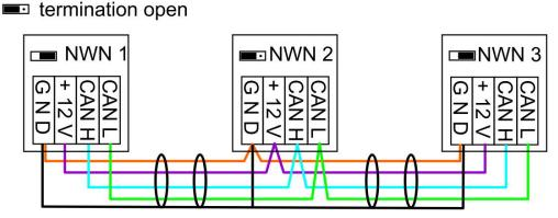
Each CAN network is to be provided with a 120 ohm BUS terminator at the first and last network subscriber (= **termination**). This is achieved with a plug-in jumper at the back of the controller. Each CAN network therefore always has two terminators (one at each end). Branch cables or a star topology are not permissible for CAN wiring.
