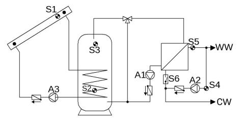
**WARNING:** The excess collector temperature limiter is activated for **A1** by default. This must be changed to **A3** or deactivated entirely.
