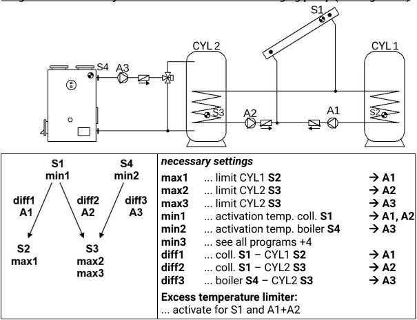
Program 192 – Solar system with 2 consumers and charging pump (heating boiler)
