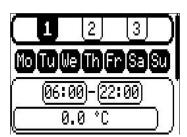
If the option **Technician level/Parameters/Time prog. set values** is set to **"Yes**", the time programs change such as to allow adjusting of said set values below the different time windows.
