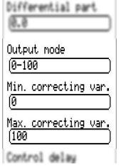
Depending on the make of the pump, the control mode of the pump can be set to normal (0-100 "solar mode", PWM 2) or inverse (100-0 "heating mode", PWM 1). There may also be specific requirements for the limits of the control range. These can be found in the information of the pump manufacturer.
