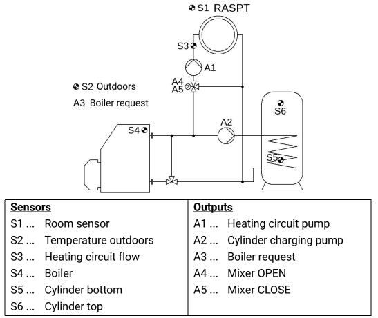
**Basic functionality (P896):** No buffer, cylinder charging pump = A2, Boiler request = A3.
