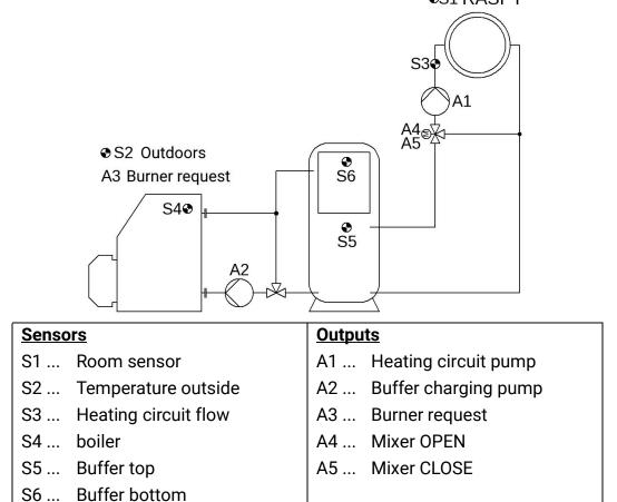
**Basic functionality (P912):** The combined buffer is held to a certain temperature by the automatic burner. Buffer charging pump **A2**, burner request **A3**, Mixer regulation **A4+A5**.
