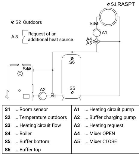
**Program 832:** Enabling of the heating circuit pump **A1** via boiler temp. and buffer temp., regulation of buffer charging pump **A2**, burner request related to buffer.
