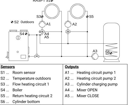
**Basic functionality (P960):** Regulation of the heating circuit pumps **A1**, **A2**, and the cylinder charging pump **A3**, mixer regulation for the first heating circuit **A4+A5**; regulation of the second heating circuit can be achieved via speed control for **A2**.
