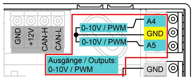
The connections A4 & A5 are the positive pole, the GND connection is the negative pole.
