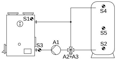
**Program 816:** Boiler circuit pump **A1** is enabled, if **S1** exceeds the threshold *min1* and **S4** is greater than **S2** by the difference *diff1* and **S2** has not exceeded the threshold *max1*.
