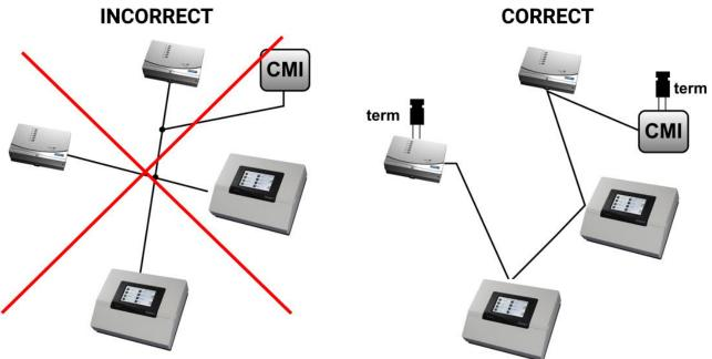
**Example:** Connection of three network nodes (NWN) with a 2x2-pole cable and termination of the terminal network nodes (network inside one building)
