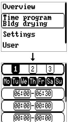
Setting up a building drying program that features time programs will cause the option **"Time program Bldg drying"** to appear in the main menu, used to parameter.
